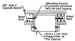
WARNOCK HERSEY UL Classified 5/8" Type X gypsum board inserted in the cavity between the two lay-LISTED ers. Warnock Hersey has approved the Safeguard Cabinets to be mounted in any face of fire rated steel or wood stud for up to 2 hour rated walls without affecting its fire rating. The above meets the requirement test ASTM-E119-98 with test report WHI-495-1534. MOUNTING INSTRUCTIONS are supplied with each safeguard cabinet.
