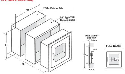
SAFEGUARD Valve Knockout Drilling: No knockouts are provided with Safeguard Valve Cabinets. Find the exact location of the pipe(s) which enter the cabinet and mark the cabinet tub appropriately. Both outside and inside tubs and insulation material must be completely open to receive pipe(s).
